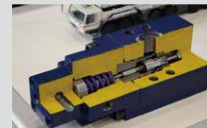
Structural Model of Pilot-assisted Hydraulic Load Control Valve (Inventors: Haibo Xie, professor; Jianbing Liu, PhD candidate; Huayong Yang, Academician)
