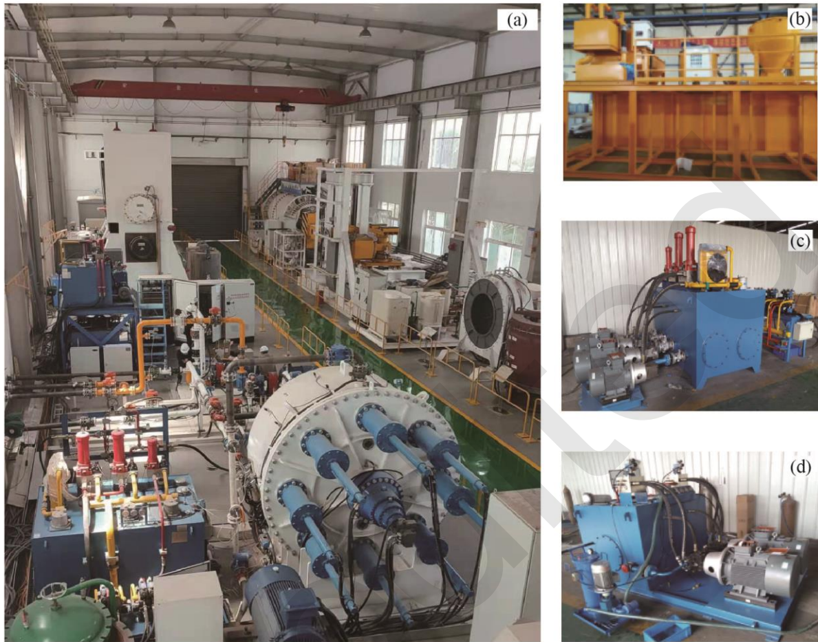
Fig. 6 Ø2.5m multi-purpose test rig for slurry shield machine: (a) overview of the test rig, (b) slurry processing, (c) hydraulic system for loading, (d) hydraulic system for driving
