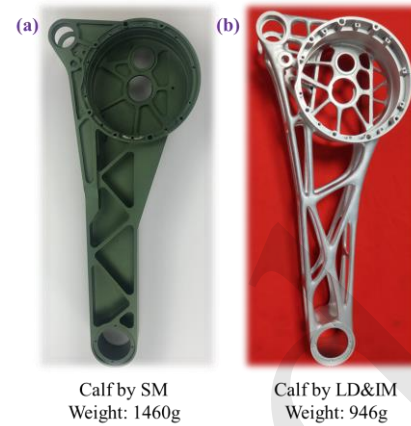
Fig. 6 More than a 35% reduction in calf weight was achieved using the LD&IM method
