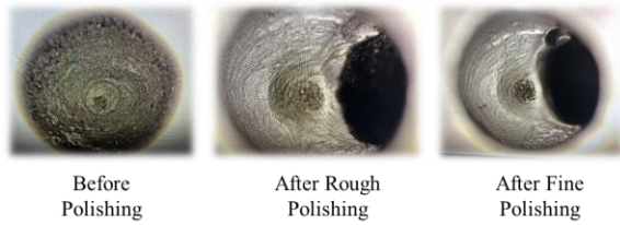
Fig. 9 Comparison of results from abrasive flow polishing
