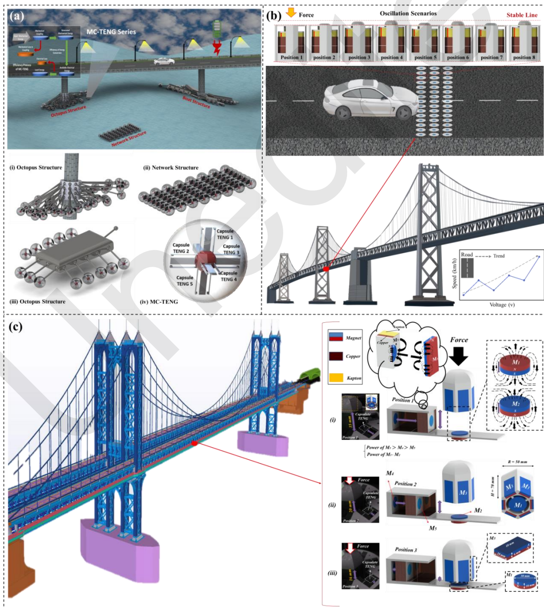
Fig.7. Magnetic Structured Triboelectric Nanogenerators for bridges: (a) Working principle of the MC-TENG (Jiao, et al., 2022b). (b) Illustration of application and various scenarios of the MCL-TENG (Jiao, et al., 2022c). (c) Design structure of the ml-TENG as a self-powered sensor (Matin Nazar, et al., 2021a)
